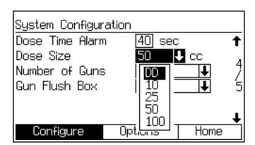
Fig. 54. Configure Screen 4, dynamic dosing selected
